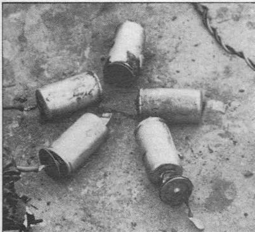
Above: the wrong way to treat a set of Ni-Cads. Readers should be aware that re-charging batteries should be done with great care. Over-charged batteries can cause serious accidents.
